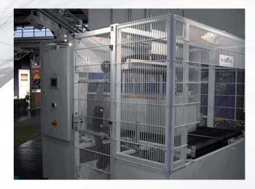
Fully automatic twist wrapping machine (plug-and-play) for all kinds of profiles and long products with low to medium production capacity.
