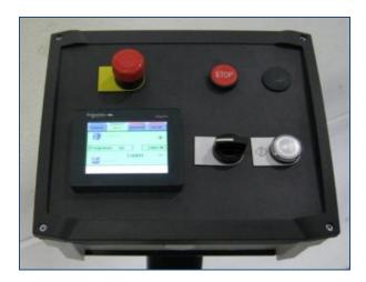
Machine HMI TFT Touschscreen panel for the operator and service team to adjust the machine and to change programme parameters
